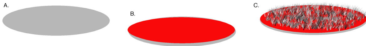
Figure 2. A) Polished ZrO 2 disc; B) Titanium coated ZrO 2 disc (Zr-Ti); C) Titanium nanotube coated Ti-ZrO 2
